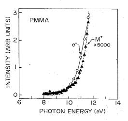
FIG. 6. Photon energy dependence of photoion and photoelectron emission from PMMA near the ionization threshold. The photon energy dependence of the incidence photon flux is included.
