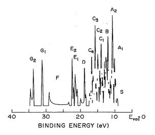
FIG. 4. VEH density of states for an isolated *s*-PMMA chain. The binding-energy scale of the DOS curve is shown after a contraction of 1.25 in energy scale and a rigid shift (2.54 eV) (see Table I for uncollected results).
