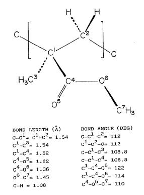
FIG. 3. Schematic representation of the structural unit cell used for VEH band-structure calculations on *s*-PMMA. The atom numbering and the geometrical parameters are shown.
