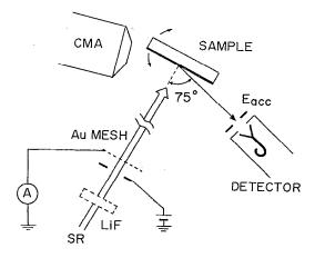
FIG. 1. Scheme for experimental setup. CMA: double-pass cylindrical mirror analyzer for photoelectron spectra.  $E_{acc}$ : electrode for electron and ion collection. A LiF filter was used for the measurements with photon energies below 12 eV to reduce the second-order light.
