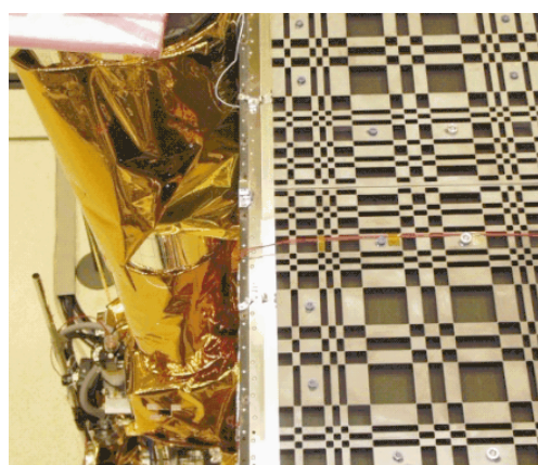
Fig. 8. the Mask in the direction of the star trackers. One of the star tracker baffle (left), covered with MLI is also visible.
