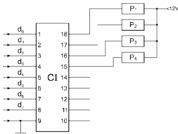
Figure 1. Electronic diagram of the interface to control the micro-pumps. CI = integrated circuit LM2803;  $d_0, d_1, \dots, d_7$  = input lines,  $P_1, P_2, P_3$  and  $P_4$  = micro-pumps.
