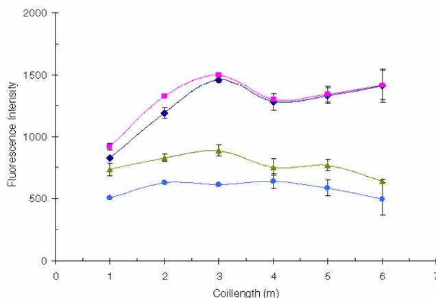
Fig. 3. Effect of the reduction coil length for different carrier flow rates on the fluorescence signals of a full cream cow milk with  $6.1 \text{ ng ml}^{-1}$  Te. In all experiences it was used a KBr concentration of 30% (w/v). Measurements were made using the multicommution approach and error bars indicate the variability ( $\pm s$ ) of three independent assays. (◆)  $3.4 \text{ ml min}^{-1}$ ; (■)  $4.6 \text{ ml min}^{-1}$ ; (▲)  $5.7 \text{ ml min}^{-1}$ ; (●)  $6.5 \text{ ml min}^{-1}$ .
