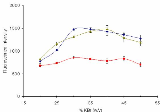
Fig. 2. Effect of KBr concentration on the fluorescence signal of total Te in a full cream milk with  $6.1 \text{ ng ml}^{-1}$  Te. In these experiments, the flow rate was fixed at  $4.6 \text{ ml min}^{-1}$ . Bars indicate the variability ( $\pm s$ ) of three independent assays using different reduction coil lengths: (■) 2 m; (◆) 3 m; (▲) 4 m.
