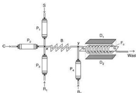
Fig. 1. Flow injection chemiluminescence system.  $P_i$ , solenoid micro-pumps;  $D_i$ ,  $100 \text{ mm}^2$  active area photodiodes; FC, 20 cm-coiled polyethylene flow cell; B, 25 cm mixing tube; *x*, *y*, confluence points; S, sample;  $\text{R}_i$ , reagents; C, carrier (water).
