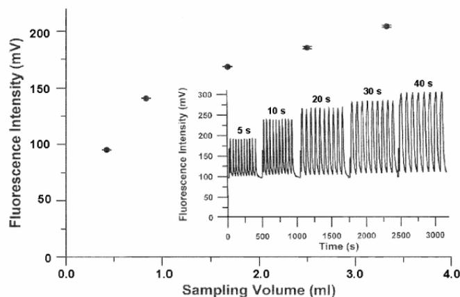
Fig. 4. Effect of sampling volume on the multicommutation AFS determination of Hg using a reduced volume liquid/gas phase separator. Hg concentration of 0.6  $\mu\text{g l}^{-1}$ . Inset: signals obtained at different sampling times (from 5 to 40 s) using a reading time of 30 s, for 5 and 10 s sampling time, and a reading time of 40 s for high sampling time intervals.
