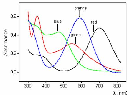
Fig. 4. Absorption spectra of the chemical products measured with indication of the LEDs emission for  $\text{Fe}^{3+}$  (blue LED) nitrite (green LED), carbaryl (orange LED) and phenol (red LED) determinations, with 470, 546, 596 and 700 nm of maximum absorbance, respectively. The arrows show the maximum emission point of the employed LEDs (466, 566, 590 and 660 nm, respectively).
