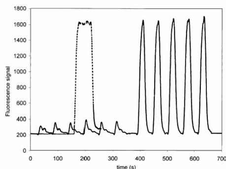
Fig. 2 Fluorescence signal of Te obtained by continuous (dashed line) and multicommutation (dashed line) modes. Te concentration =  $3 \text{ ng mL}^{-1}$ . When using the continuous system, one signal was presented. Using multicommutation mode six blanks and five signals were obtained, measured in lower sensitivity range than that used for continuous measurements
