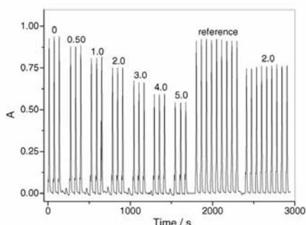
Fig. 3. Transient signals obtained for different solutions of sodium cyclamate. Numbers indicate concentrations in  $\text{mmol L}^{-1}$ .
