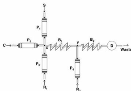
Fig. 1. Multicommutated flow-system for cyclamate determination. P<sub>1</sub>, solenoid micro-pumps; D, spectrophotometric detector (350 nm); B<sub>1</sub>, B<sub>2</sub>, coiled reactors (100 and 50 cm); x, y, confluence points; S, sample; R<sub>1</sub>, 0.20 mmol L<sup>-1</sup> NaNO<sub>2</sub>, R<sub>2</sub>, 0.20 mol L<sup>-1</sup> KI; C, carrier (0.1 mol L<sup>-1</sup> H<sub>3</sub>PO<sub>4</sub>).
