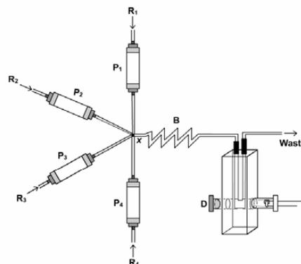
Figure 3. Flow diagram of the system. *P*<sub>1</sub>, *P*<sub>2</sub>, *P*<sub>3</sub> and *P*<sub>4</sub> = solenoid micro-pumps; *R*<sub>1</sub>, *R*<sub>2</sub>, *R*<sub>3</sub> and *R*<sub>4</sub> = sample and reagent solutions, (for details see text); *x* = joint device; *B* = reactor coil, 120 cm length and 0.8 mm i. d.; *D* = mortise to fit the photodiode.
