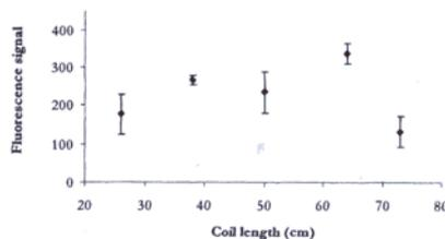
**Figure 3. Effect of the reaction coil length on the fluorescence signal for a bismuth concentration of 8.4 ng/mL. Measurements made by multicommutation HG-AFS with a sample flow rate of 4.6 mL/min, NaBH<sub>4</sub> flow rate of 5.0 mL/min, and blank flow rate of 5.0 mL/min.**
