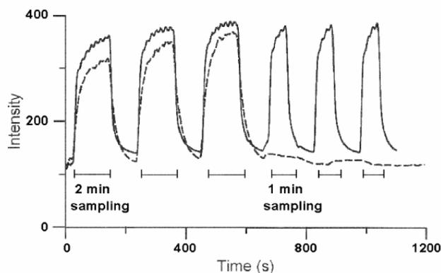
Fig. 3. Effect of the argon flow on the Hg AFS signal profile (—), use of Ar for liquid/gas phase separation in continuous operation mode; (---), use of Ar as gas phase carrier in multicommutation mode. Hg concentration employed was  $1 \mu\text{g l}^{-1}$ . When using the continuous system, three signals and three blanks were presented. Using Ar as carrier in the multicommutation mode three signals were obtained for 2 and 1 min sampling times, respectively.
