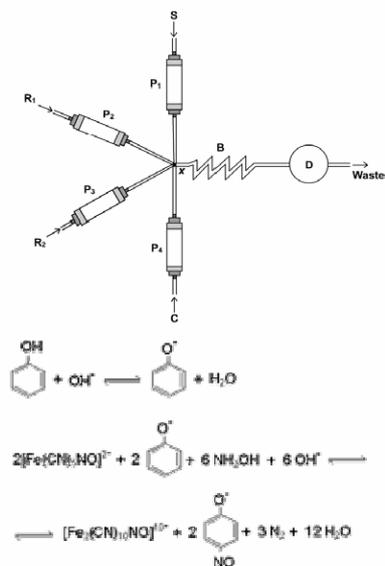
Fig. 1 Multicommutated flow manifold diagram. S – sample or standard solution; R<sub>1</sub> – 3.0 × 10<sup>-2</sup> mol L<sup>-1</sup> sodium nitroprusside solution; R<sub>2</sub> – 3.0 × 10<sup>-2</sup> mol L<sup>-1</sup> hydroxylamine hydrochloride solution; C – carrier buffer solution, pH 12.3; P<sub>1</sub> – solenoid micro-pumps; x – confluence point; B – 100 cm mixing tube 0.8 mm i.d.; D – detector.
