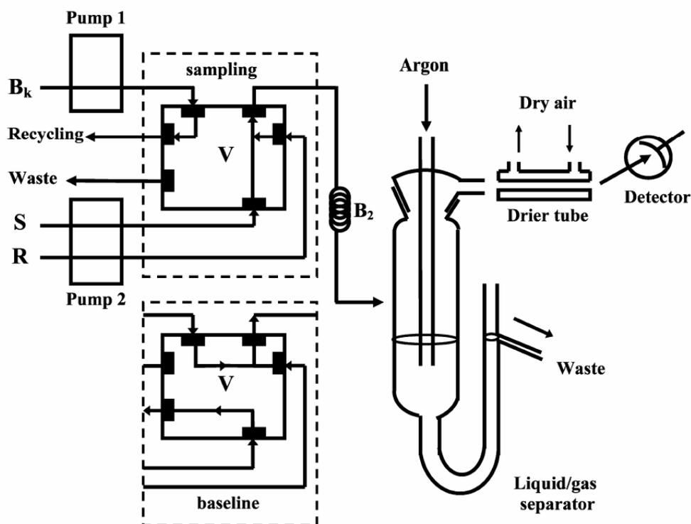
Fig. 1. Manifold employed to operate AFS in the continuous mode. R, reductant reagent; B<sub>k</sub>, blank solution; S, standard solution; V, sampling valve; B<sub>2</sub>, reaction coil. The scheme indicates the two positions of the mixing valve incorporated to control alternatively the sample or standard fluorescence and the baseline.
