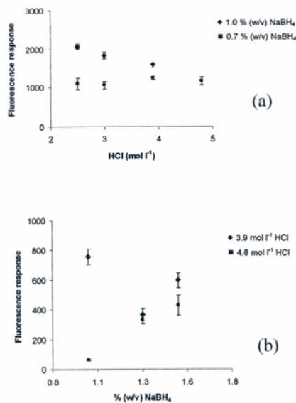
Figure 4. Effects of NaBH<sub>4</sub> and HCl concentrations on bismuth determination by HG-AFS using (a) continuous and (b) multicommutation modes.
