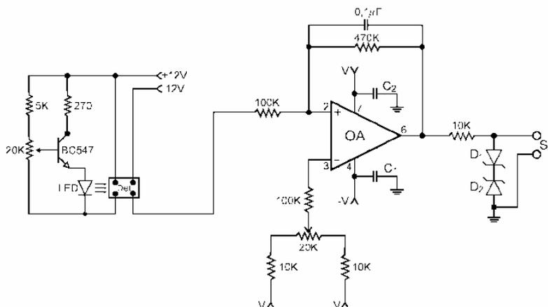
Figure 2. Diagram of the photometer. Det = Photodiode, RS 10530 DAL; OA = Operational amplifier, OP07; C<sub>1</sub> and C<sub>2</sub> = Tantalum capacitor, 1  $\mu$ F; D<sub>1</sub> and D<sub>2</sub> = Zener diode, 4.5 V; and S<sub>0</sub> = output signal.
