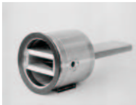
Figure 6.3: An SPS pick-up installed in the beam pipe.
