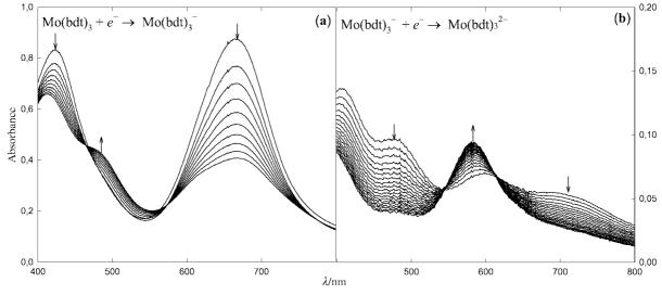
Fig. 1 Repetitive diode-array UV-scans from reaction mixtures in dry THF containing: (a) Mo(bdt)<sub>3</sub> 3.38 × 10<sup>-5</sup> mol dm<sup>-3</sup> and n-Bu<sub>4</sub>NOH 3.38 × 10<sup>-5</sup> mol dm<sup>-3</sup> (spectra taken every 0.2 s, shown every 1 s, T = 300.2 K). (b) Mo(bdt)<sub>3</sub>-  $1.16 \times 10^{-5}$  mol dm<sup>-3</sup>, n-Bu<sub>4</sub>NOH  $3.28 \times 10^{-4}$  mol dm<sup>-3</sup> (spectra taken every 0.5 s, shown every 10 s, T = 301.2 K).
