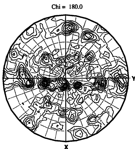
Figure 3. Representation of the X=180^\circ section of the self-rotation function from the P. aeruginosa NAGK crystals. Start level at 1\sigma and step size of 0.75\sigma . The orthogonalization code follows the PDB convention. See text for interpretation.
