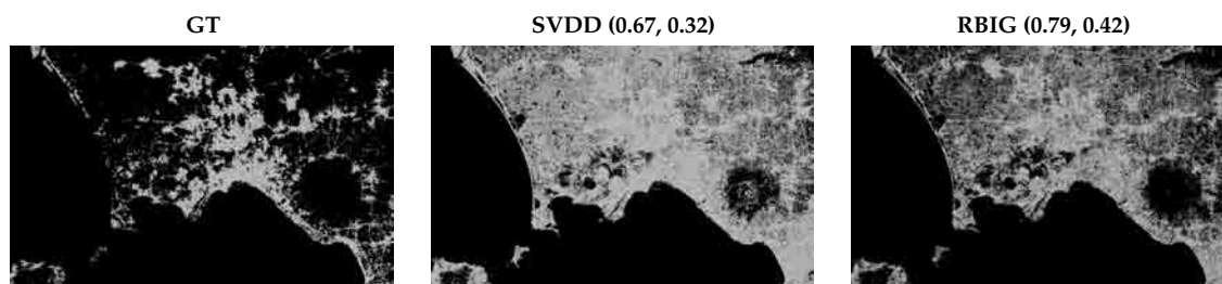
Figure 5.21: Ground-truth (GT) and classification maps obtained with SVDD and RBIG for the Naples 1995 scene. The white points represent urban area and the black points represent non-urban area. The corresponding overall accuracy and \kappa -statistic are given in parenthesis.
