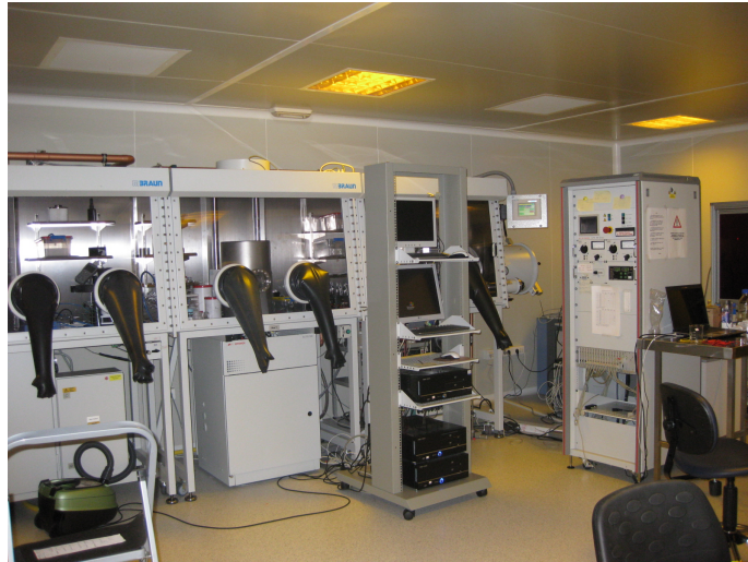
Figure 1.7: clean-room of the class ISO 7 10000 with glove box, located in the Instituto de Ciencia Molecular (ICMOL) in Valencia.
