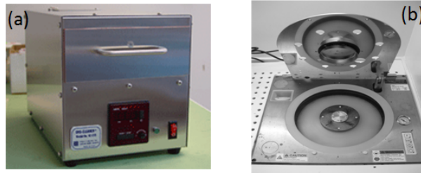
Figure 1.8: Picture of (a) the UV-Ozone cleaning device and of (b) the Suss Micro Tec spin coating system.
