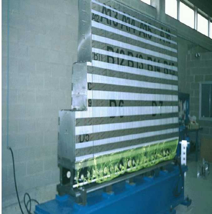
Figure 2.13: A Tile Calorimeter extended barrel module constructed in Spain.
