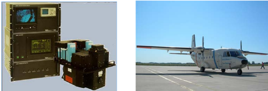
Figure 3.2. AHS sensor. Scan-head and operator console and INTA C-212-200 EC-DUQ airplane.
