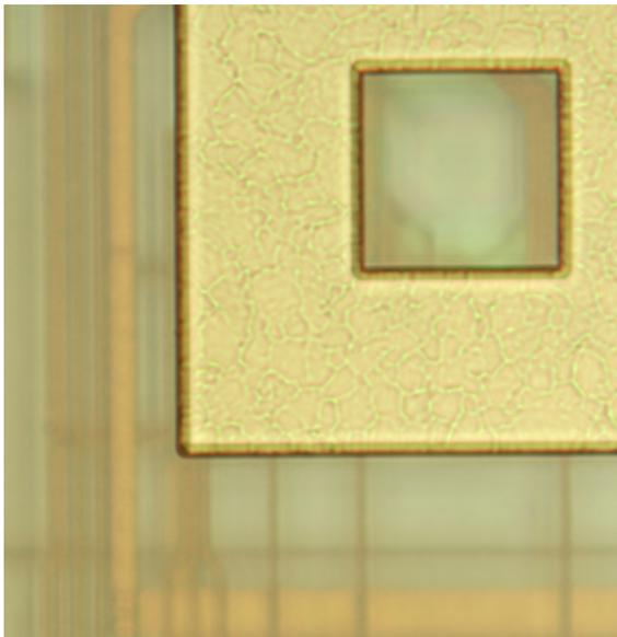
(b) Detail of the fourth metal layer covering the whole pixel matrix. Only the photodiodes are exposed to incident light.
