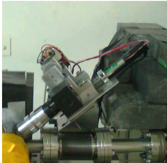
Figure 3.20: Focus system. It moves the whole optical system closer to the target or away in the 40 degree direction with respect to the beam.
