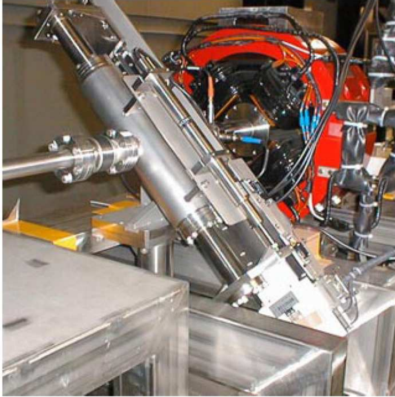
Figure 2.15: WS as installed in ATF2. The stage moves in 45^\circ direction.
