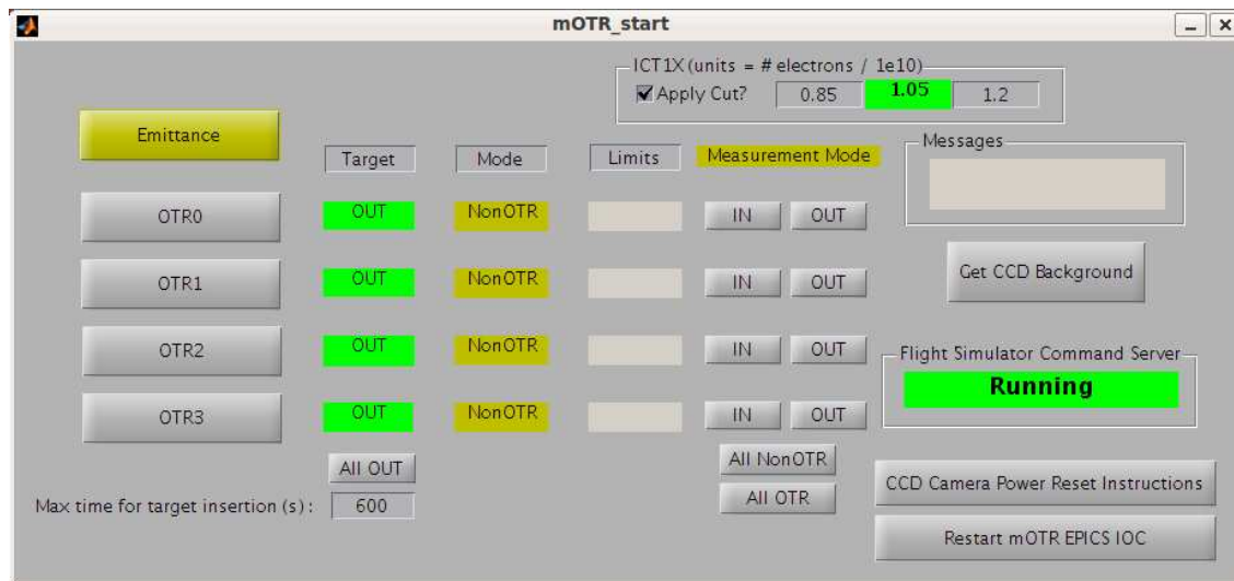
Figure 3.26: Main Panel of the Multi-OTR GUI. It is opened from the main menu in the ATF2 control room.
