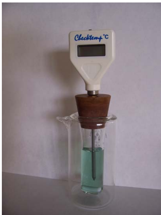
Figure 1. Photograph of the calorimeter containing 20 mL of a colored solution for the sake of viewing.
