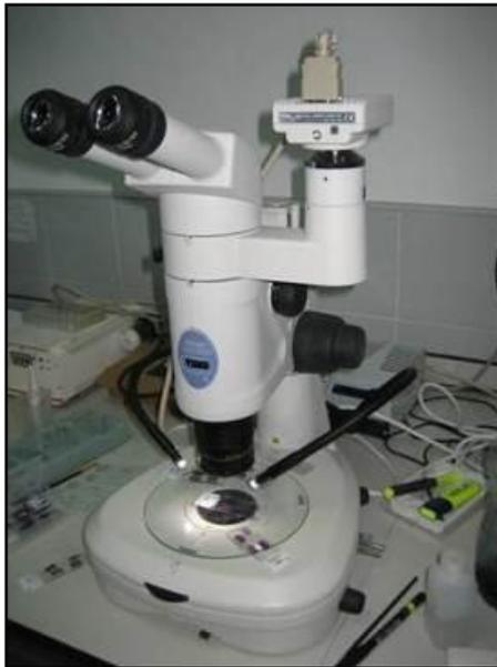
**Fig. III.15.** Microscopio NIKON SMZ 1500
