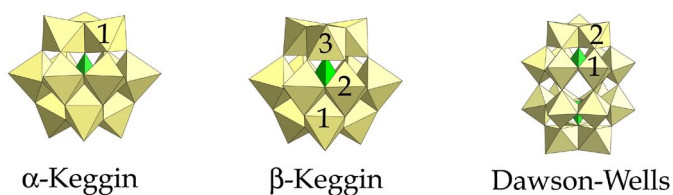
Figure 3. \alpha -( T_d ) and \beta -( C_{3v} ) isomers of the [\text{SiW}_{12}\text{O}_{40}]^{4-} and \alpha\text{-}[\text{P}_2\text{W}_{18}\text{O}_{62}]^{6-} . The number in the figure represents the octahedron removed to give each vacant isomer.
