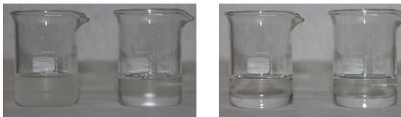
Figure 7.8 Pictures of the micellar solution (a) before and (b) after micelle formation upon stirring showing the difference in transparency.
