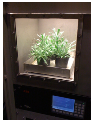
Figure 10. Gas chamber for incubation of plants with 13 CO 2 .
