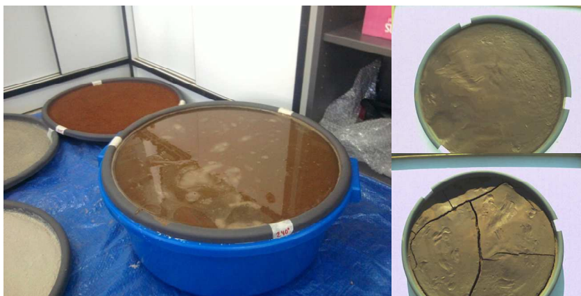
Figure 2.4 Saturation process of an IBS sample. During drying some silt and clayey samples presented cracks.
