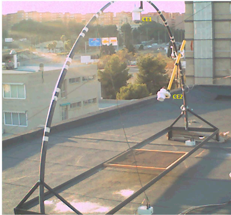
Figure 2. Experimental ensemble used in the study during two simultaneous measurements at nadir (CE1) and at zenithal angle (CE2).
