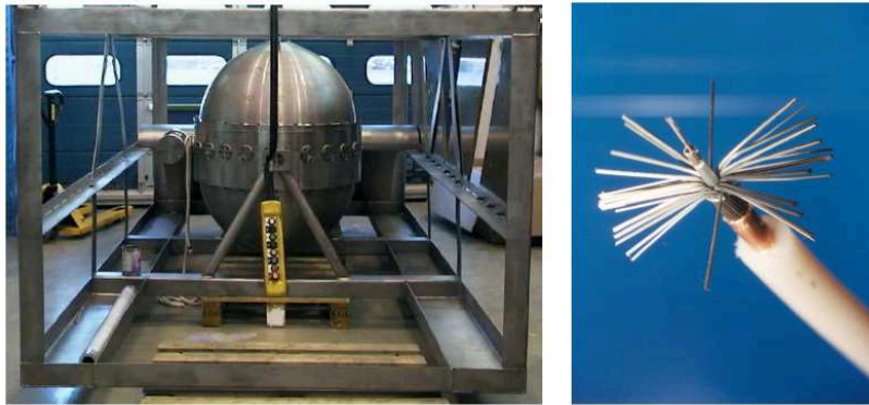
Figure 2.12: Pictures of the junction box vessel with its frame (left) and of the main electro-optical cable (right).
