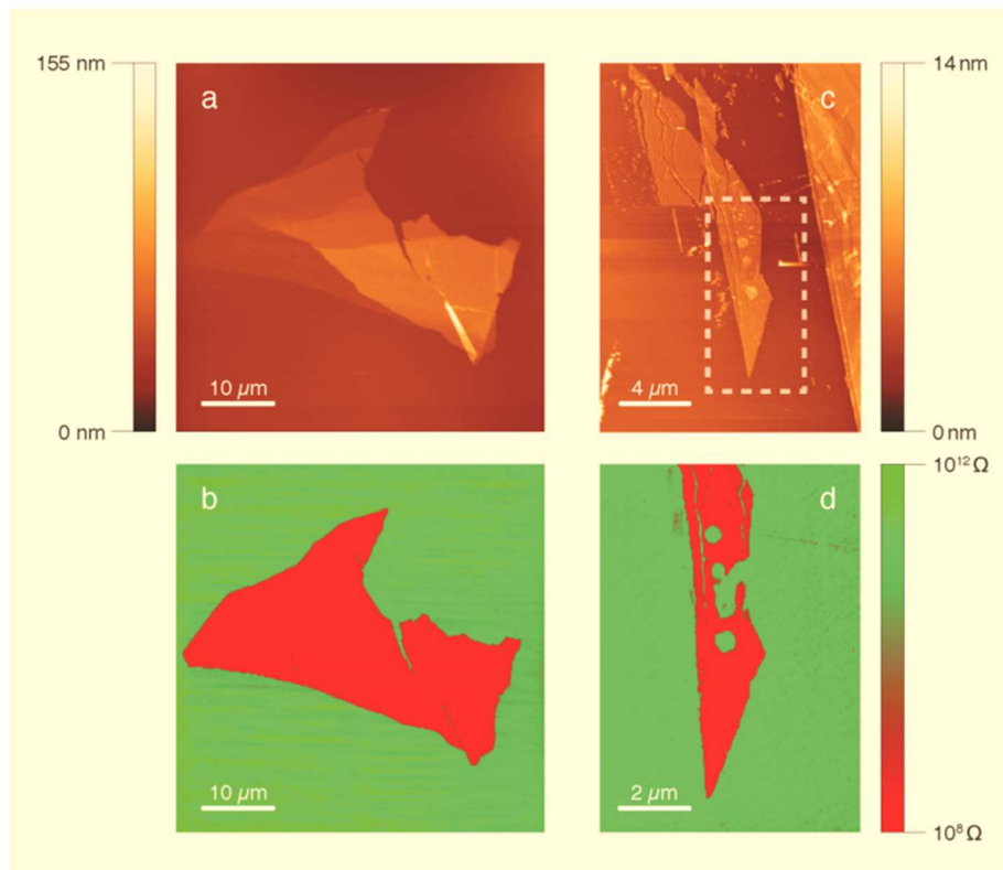
Figure 28. (a) AFM topography image measured in contact mode of a TaS 2 flake. (b) CT-AFM resistance mapping of the same flake. (c) AFM topography image of TaS 2 thin flakes. The flake inside the dashed box has been patterned with three round oxidized regions. (d) CT-AFM resistance mapping of the patterned flake highlighted in (c).
