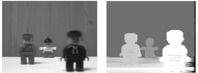
Fig. 4. EI with shallow DOF captured with SAIL method (Left). Disparity map for the EI on the left (Right).
