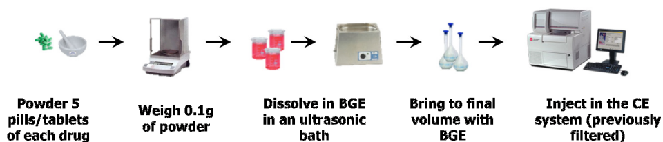
Figure IV.8: Scheme of the experimental procedure used for the chiral analysis of fluoxetine in pharmaceutical formulations by EKC-CFT.
