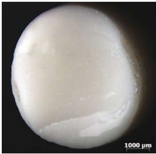
Fig. 2. Representative image of the predominantly cohesive fracture of the infrastructure for the lithium disilicate (LD) groups visualized under optical microscopy.
