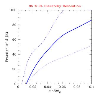
FIG. 10: Sensitivity to  $sgn(\Delta m_{31}^2)$  for different values of  $|\Delta m_{31}^2| = 2.0 \times 10^{-3} \text{ eV}^2$  (dotted line),  $2.4 \times 10^{-3} \text{ eV}^2$  (solid line), and  $3.0 \times 10^{-3} \text{ eV}^2$  (dashed line). We have exploited the data from two off-axis detectors located at 200 km and 810 km by assuming ScI with a 25 kton water-Čerenkov detector at the near site and the proposed NOvA detector at the far site.
