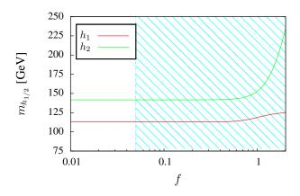
FIG. 3: One-loop masses of the two lightest Higgs bosons as functions of f. The values of all the other parameters are given in the text. The shaded area is excluded by  $\mu \to e\gamma$ .
