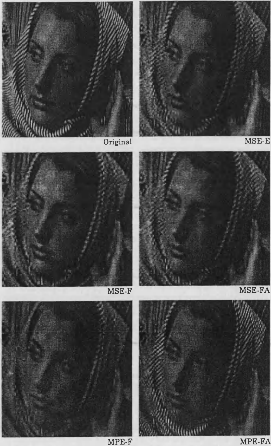
Fig. 5. Compression results on Barbara image (0.5 bpp). The figures show the 170 × 170 central subimage.
