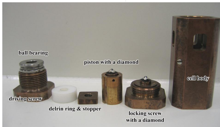
Figure 3.6: Up: Vertical cross section of the DAC for PPMS. Down: DAC components.[99]
