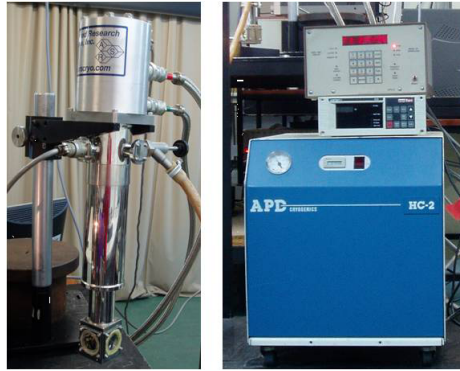
Figure 3.10: Closed-cycle helium cryostat components (left) and compressor (right) used for low temperature experiments down to 15 K.
