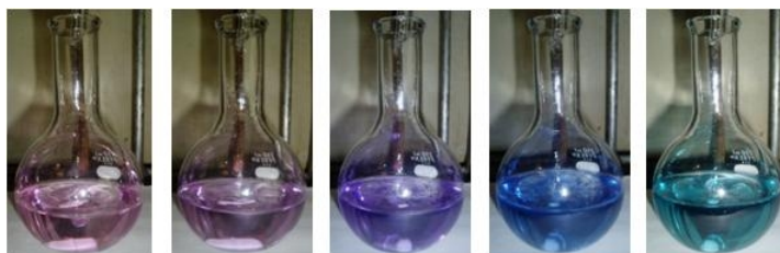
Figure 7.1: Preparation of \text{ZnO}:\text{Co}^{2+} colloidal nanocrystals in the department of Chemistry at the University of Washington. The solution change from pink to blue indicates the conversion of octahedral \text{Co}^{2+} to tetrahedral \text{Co}^{2+} .
