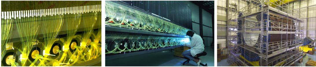
Figure 4.2: TileCal sub-detector is made in a sandwich-like structure where scintillator tiles are placed between metal sheets. On the left, photo of the WLS fiber bundles. In the center the image of the fibers during assembly. On the right a whole view of the assembly of the TileCal.
