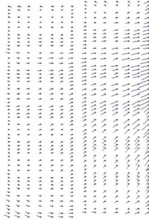
Figure 3.16: Example of spatial distortion map in one TPC computed using laser data. The arrows indicate the displacement appearing when turning on the magnetic field, magnified by a factor of 10. Figure from [95].
