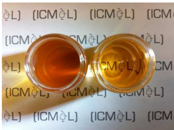
Figure 3.14- Picture showing the appearance of an orange-brown sediment in the vessel of the electrochemical cell after temporal evolution of the electrolyte. The right vessel shows the fresh electrolyte and the left vessel the result of 24 hours evolution.
