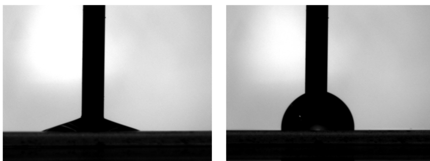
Figure 8.6- Contact angle measurement of a water droplet on the clean LSMO substrate ( left ) and after the LB deposition of the molecular monolayer of N965 ( right ).
