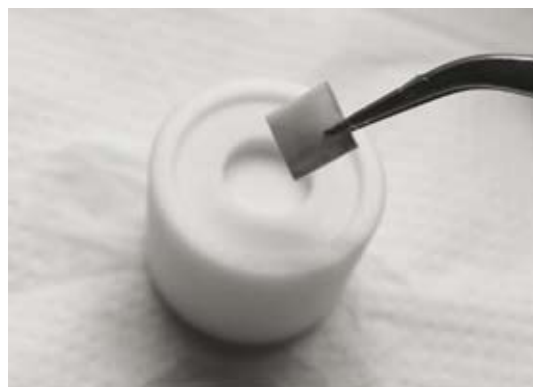
Fig. 1. The specimens placed in a Teflon sample holder made for the tooth block size.
