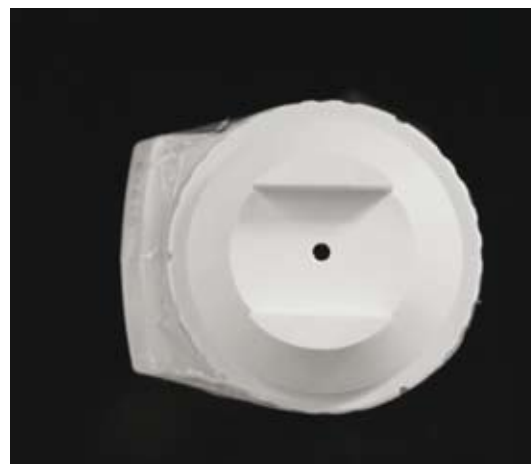
Fig. 3. Illumination/reading area of the SAV of 3 mm.
