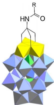
Figure 6. Representation of tris-alkoxo functionalization of Dawson-Wells structure [\text{R-CONH-C}(\text{CH}_2\text{O})_3\text{P}_2\text{V}_3\text{W}_{15}\text{O}_{59}]^{6-} . \text{VO}_4 yellow, \text{WO}_4 blue, \text{PO}_4 green.
