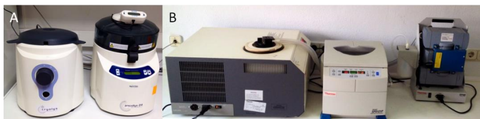
Figure 2.1. A) Precellys 24 Dual equipped with a Cryolys cooler. B) Savant SpeedVac connected to an oil-free vacuum pump and a refrigerated vapor trap.
