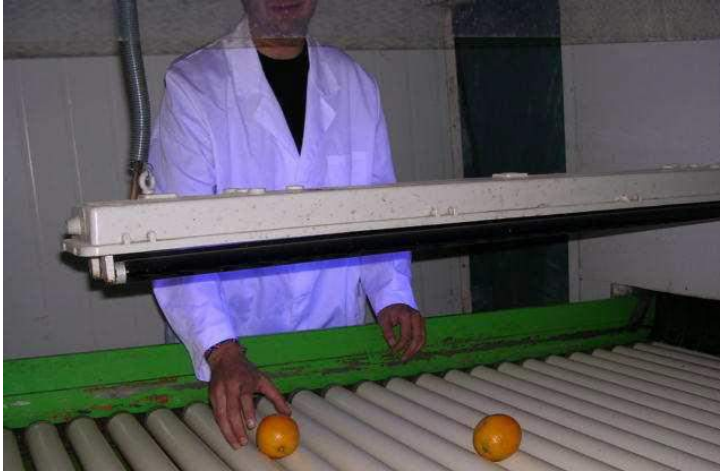
Figure 1.2. Operator examining citrus fruit under UV light to detect possible decay in a commercial packinghouse.
