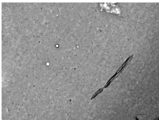
Figure 2. TEM micrograph of PLA-BCNW films containing 1 wt.% BCNW. Scale marker correspond to 2 µm.
