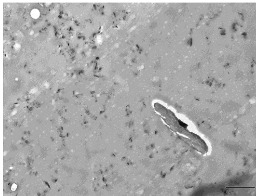
Figure 2. TEM micrographs of PHBV-BCNW films containing 1 wt.% BCNW. Scale markers correspond to 2 \mu m.
