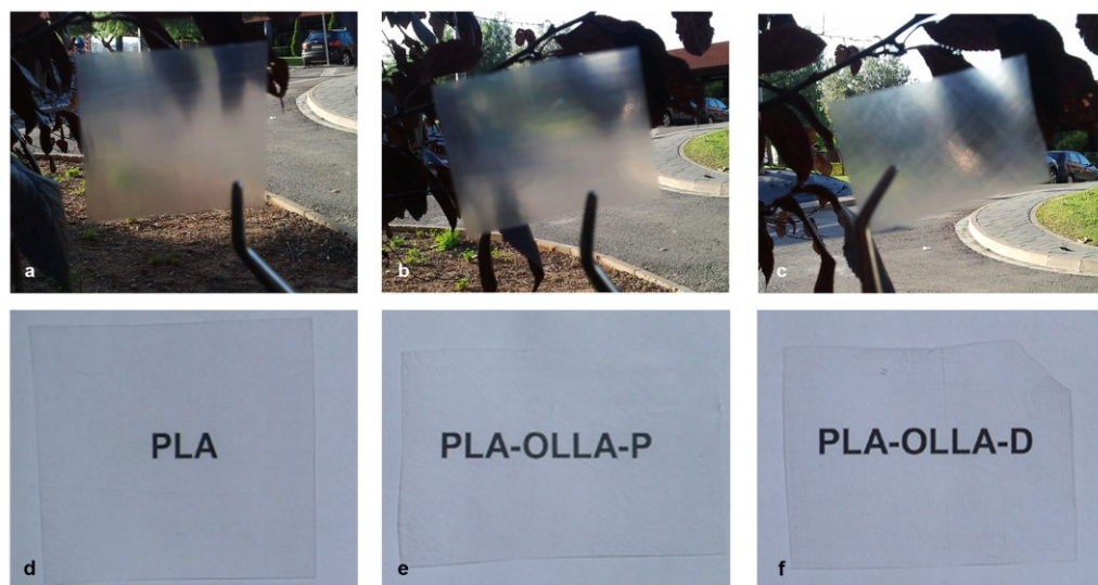
Figure 3. Photographs of \sim 100\mu\text{m} thickness films showing their transparency against a background and contact transparency, respectively, for PLA (a, d), PLA-OLLA-P (b, e) and PLA-OLLA-D (c, f)
