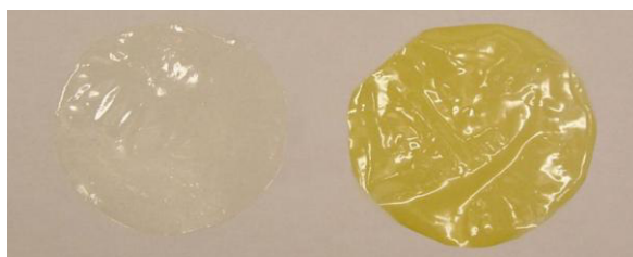
Figure 4.4.2. CS-CD-35G composites conditioned at 75% RH, before (left) and after (right) in contact with carvacrol for three months.
