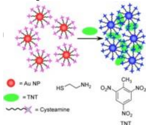
Figure 10: Assay for direct colorimetric visualization of TNT based on the D-A interaction between TNT and cysteamine at the AuNP solution interface.
