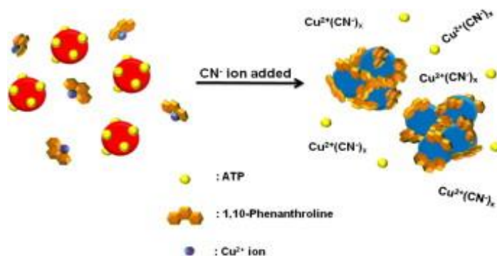
Figure 9: Schematic representation of colorimetric sensing of cyanide anion in aqueous solution employing triphosphate stabilized AuNPs.
