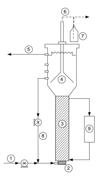
**Fig 1** Schematic diagram of the laboratory scale EGSB reactors used in this study. 1, feed; 2, glass balls; 3, effective volume; 4, gas-liquid-solid separator; 5, effluent from EGSB reactor; 6, biogas; 7, gas seal; 8, effluent recirculation; 9, cooling/heating bath circulator
