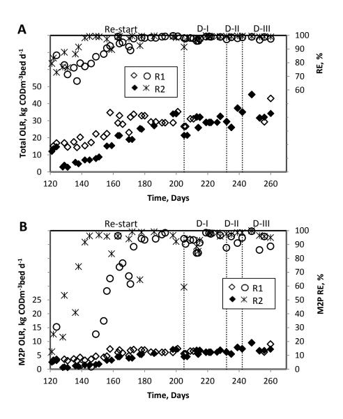
**Fig 4** Evolution of the performance of both reactors under intermittent wastewater supply. (a) Total OLR and COD removal efficiency; (b) M2P OLR and M2P removal efficiency
