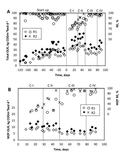
**Fig 2** Evolution of the performance of both reactors (R1 and R2) under continuous wastewater supply. (a) total OLR and COD removal efficiency; (b) M2P OLR and M2P removal efficiency
