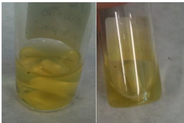
Figure 8. Stability of the palladium(II) oxamate-containing complexes after 90 days in water.
