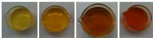
Figure 1. Bathochromic effect of the alkaline metal ion [M = Na(I), K(I), Rb(I) and Cs(I) (from left to right)] in the aqueous solutions of the [Pd(2,6-Me_2pma)_2]^{2-} complex.
