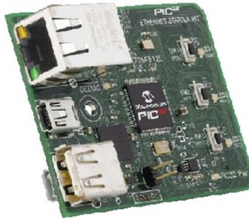
Figura 144. Tarjeta MICROCHIP DM320004 PIC32 Ethernet Starter Kit
