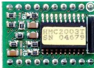
Figura 18. Sensor Honeywell HMC2003 (Honeywell 2011)
