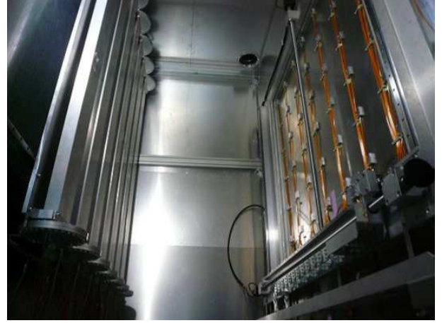
Figure 8: Photograph of the muon monitor inside the support enclosure. The silicon PIN photodiode array is on the right side and the ionization chamber array is on the left side. The muon beam enters from the left side.
