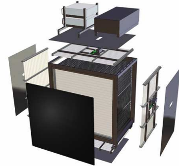
Figure 13: The Proton Module. Similar to the INGRID modules, but with finer grain scintillator and without the iron plates.
