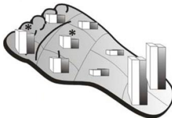
Figure 25. Example of a representation of the mean peak pressure during Walking (white) and Nordic Walking (grey) (adapted from (Pérez-Soriano et al., 2011)).
