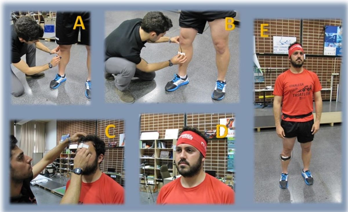
Figure 58. Accelerometer placement protocol: A) Shaving the location; B) Placing the tibial accelerometer; C) Placing the head accelerometer; D) Securing the head accelerometer; E) Whole-body view.
