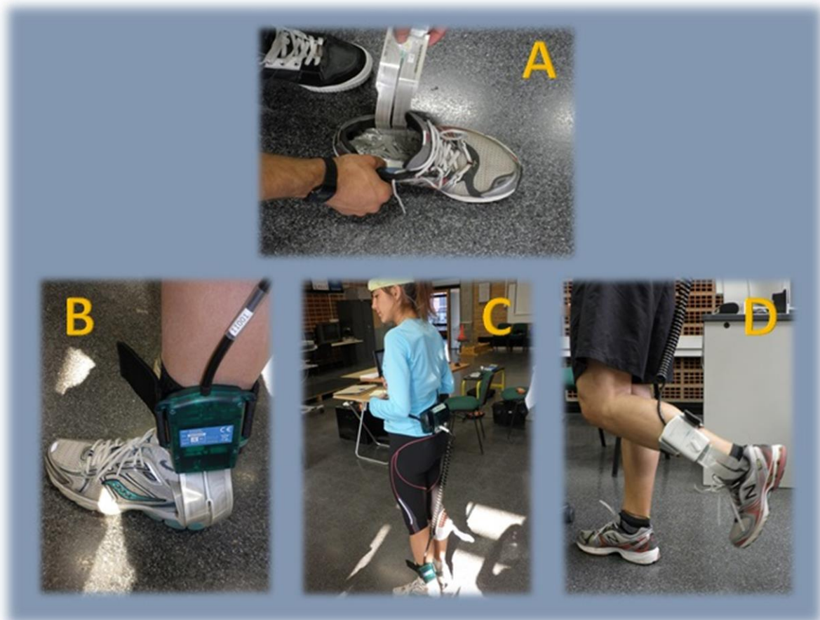
Figure 55. Calibration process for the Biofoot 2001® Pressure Analysis System. A) Inserting instrumented insole; B) Connecting instrumented insole to amplifier; C) Amplifier connected to telemetry transmitter; D) Calibration of the system.
