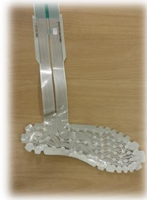
Figure 21. Array of sensors embedded into the instrumented insole.
