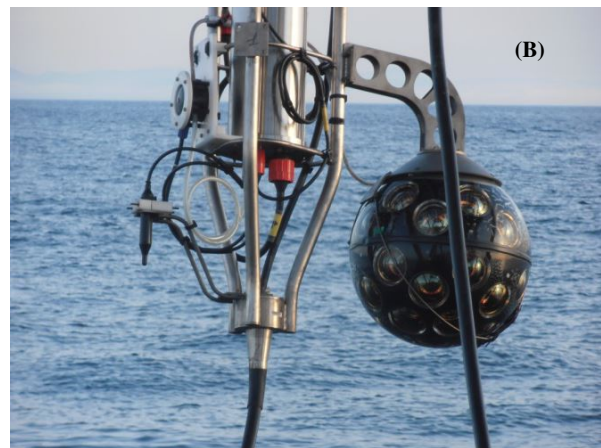
Fig. 1 (A) A 3D cutout drawing of the DOM. The zenith angle \theta and the azimuthal angle \phi are indicated. Vertically upward corresponds to \theta = 0^\circ whereas \phi = 0^\circ points to the support cable. (B) The DOM connected to the ANTARES instrumentation line. The structure to which the DOM is connected is a standard ANTARES support frame including a cylindrical electronics container.
