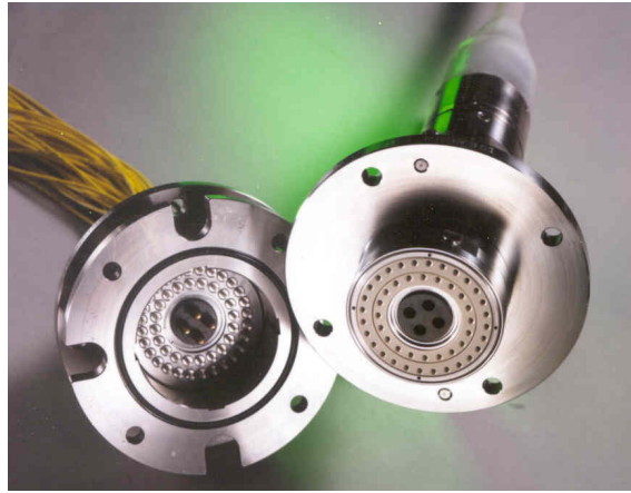
Figure 30: Electro-optical plug and receptacle for connection of the undersea cable to the junction box.
