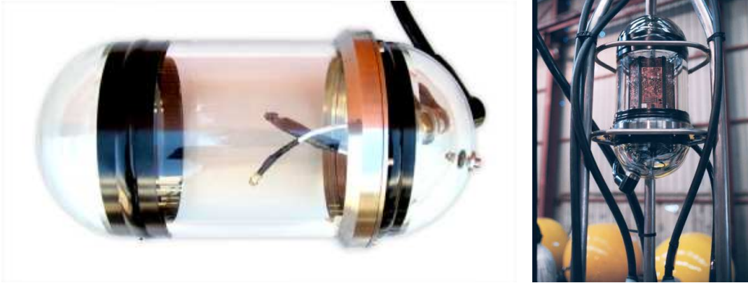
Fig. 5. Left: Example of a borosilicate glass container that houses the LED Beacons. Right: LED Beacon mounted in the Optical Module Frame.
