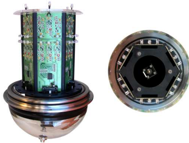
Fig. 1. An LED Beacon as viewed from sideways (left) and from the top (right). Six faces each containing six LEDs are arranged on an hexagonal cylinder. The internal photomultiplier tube is mounted at the centre of the lightguide.
