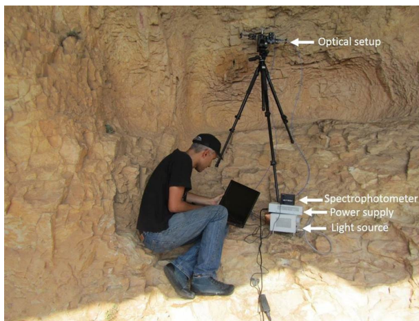
Figure 4. MFS setup used to evaluate the light stability of pigments in Cova Remígia
