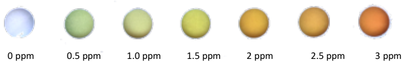
Figure S.10. Picture of the color changes observed in the film in the presence of increasing amounts of NO 2 gas.
