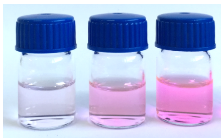
Figure 4: Visual changes observed for NM1 in acetonitrile suspension before and after exposure to 0.25 and 0.5 ppm of NO 2 gas, respectively.
