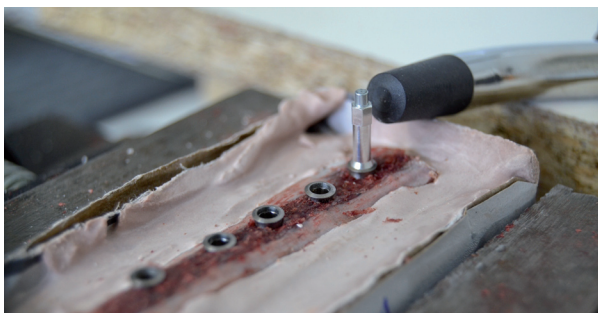
Fig. 3. Implant primary stability measured with resonance frequency analysis (Osstell ISQ).
