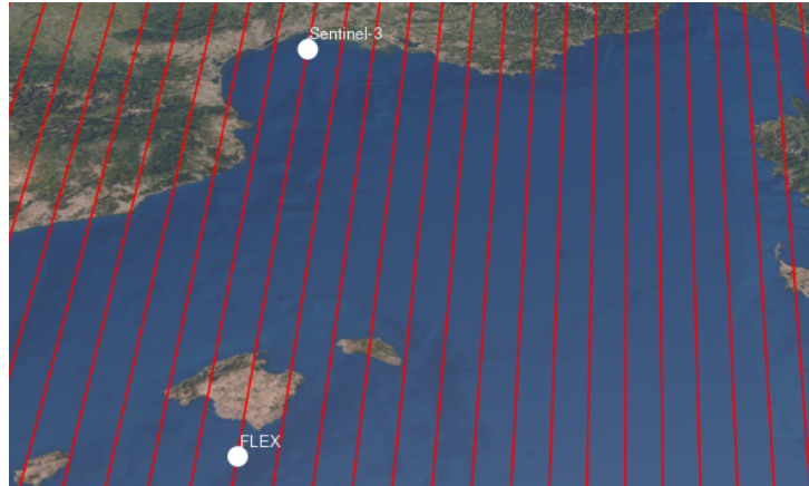
Figure 4.2: Representation of FLEX and S3 orbits based on the used external orbit data files. FLEX flies 6 s ahead of S3 in a descending Sun-synchronous orbit of 27-days repeat cycle.
