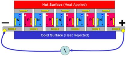
Thermoelectric Generator (TEG)
